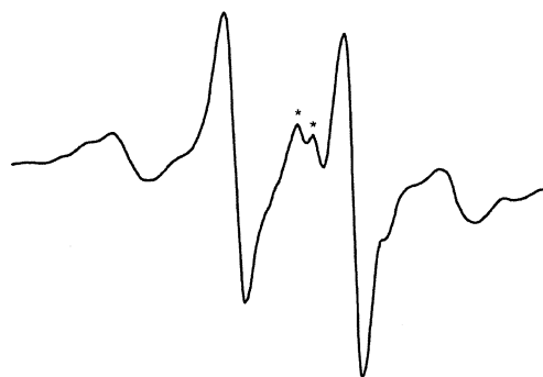
Figure 6. ESR spectrum of the surface-grafted methyl acrylate radicals ( a(H_\alpha) \approx a(H_\beta) = 19.5 G) formed in the reaction with \equiv\text{Si}^\bullet radical sites. The peaks labeled with an asterisk are due to the volume trapped \equiv\text{Si}^\bullet radicals ( g_\perp = 2.0003 , g_\parallel = 2.0018 ).
